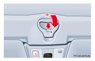
Press lock button (9) and fold down locking handle (10).
